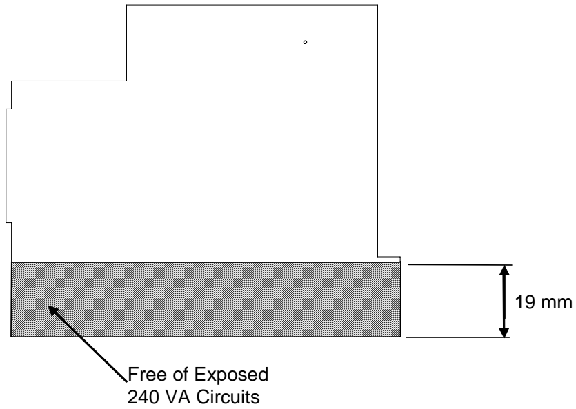
Figure 3.12. Small Form Factor I/O Expansion Card (SFF EC) – top view – 240 VA circuit keep-out area
